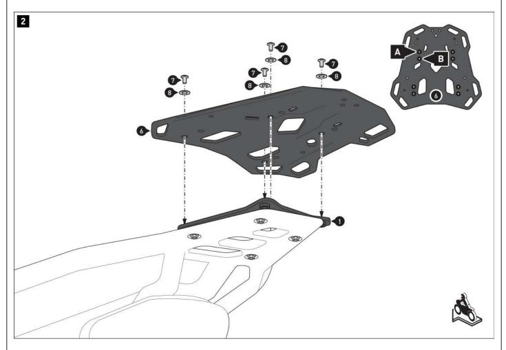
$\triangle$  **NOTE:** Depending on the space available, screw the rack (6) to the marked mounting position **(A)** or **(B)** as shown in the detailed drawing.
