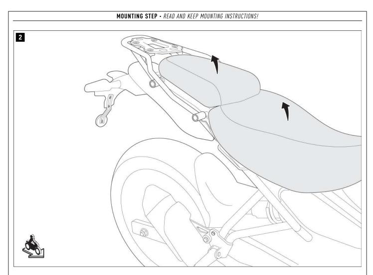
Remove the passenger seat and seat from the vehicle.
