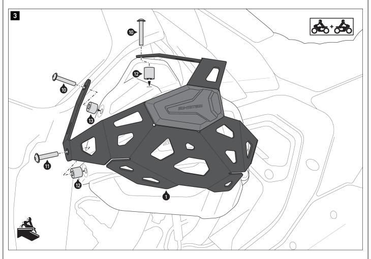
Screw the mounting bracket (1) to the **left** cylinder and the mounting bracket (2) to the**right** cylinder.
