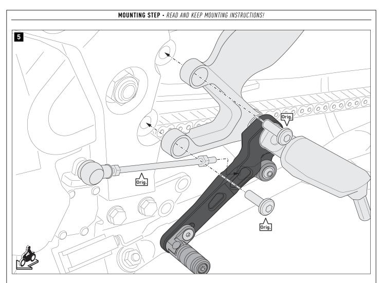
Reinstall the footrest system on the bike. A NOTE: Make sure to install the original threaded rod correctly (left-hand thread on the gear lever and right-hand thread on the bike). A WARNING: Use liquid threadlocker. Tighten the original screws (Orig.) according to the vehicle manufacturer's specifications.
