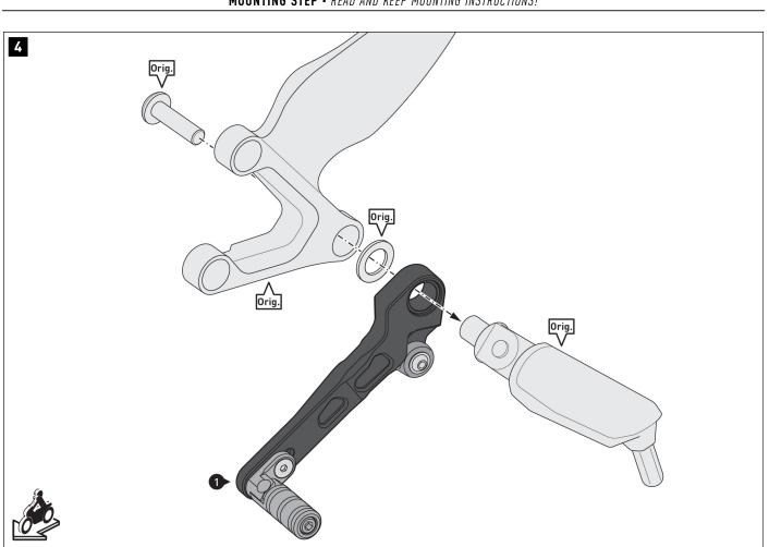
Screw the gear lever (1) onto the footrest system. A WARNING: Use liquid thread locker! Tighten the original screw (Orig.) according to the vehicle manufacturer's specifications.
