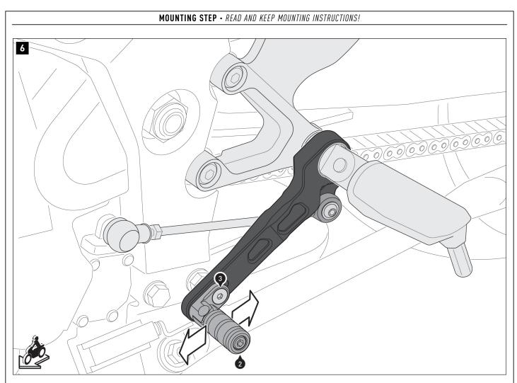
Adjust the tread (2) according to your driving habits. Tighten the screw (3) as specified in the mounting instructions.
