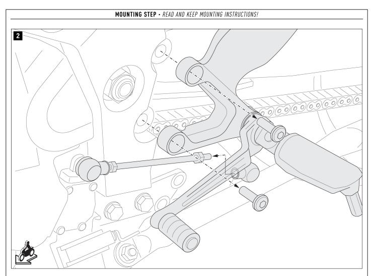
Loosen the screws shown, and remove the left footrest system from the bike.
