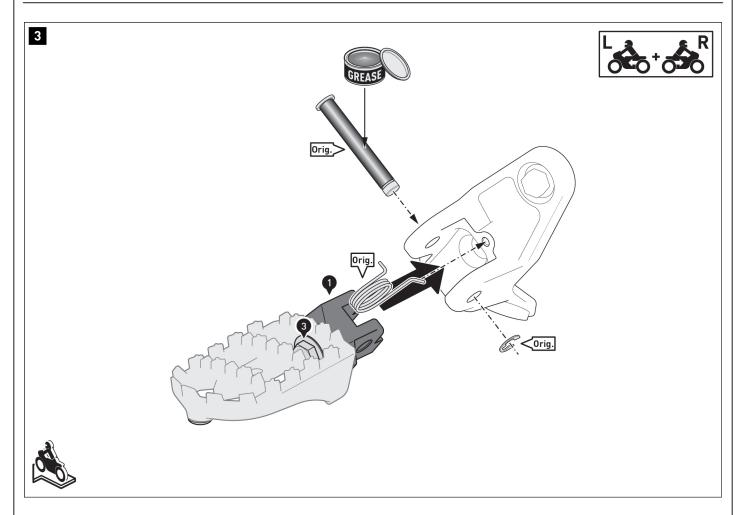
Clean the footrest mounts thoroughly. Apply rolling bearing grease to the original bolts (Orig.).
