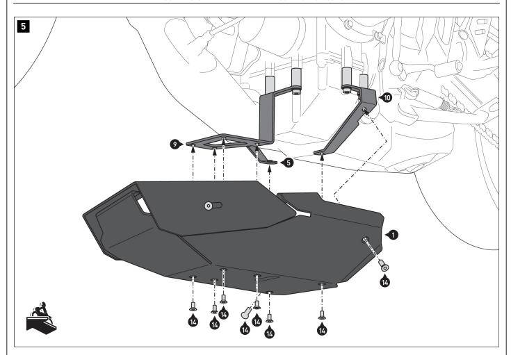
Screw the front spoiler (1) to mounting plates (5), (9), and (10). **A WARNING:** Use a liquid threadlocker!
