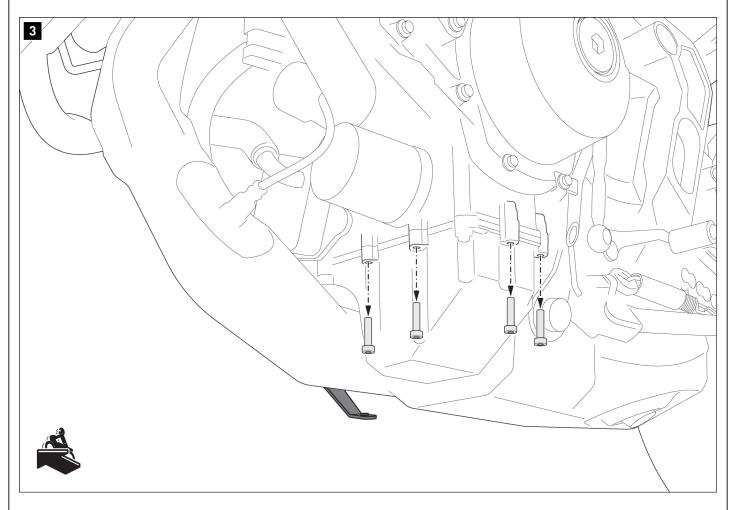
Remove the screws shown on the **left** side of the vehicle.
