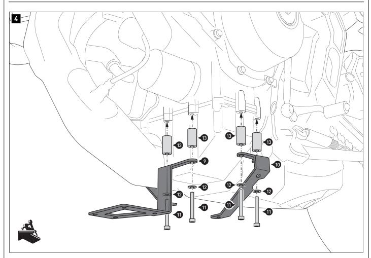
Screw mounting plates [9] and [10] onto the vehicle.
