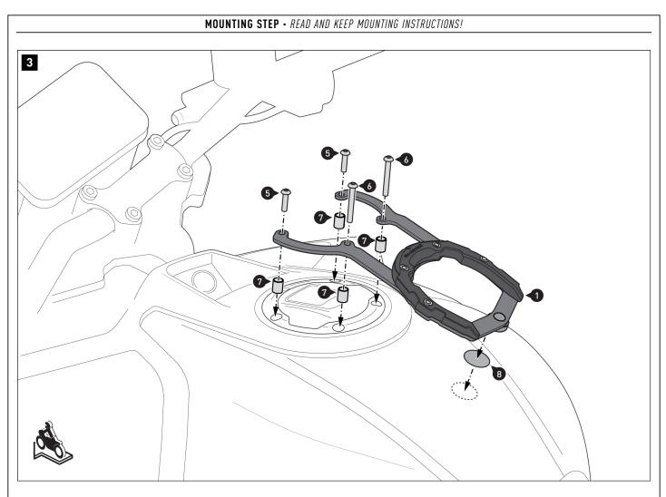
Carefully clean the surface of the tank so it's free of dirt and grease residue. Determine the support point of the vibration dampener [4]. Then stick the adhesive protective foil (8) onto the support point.
