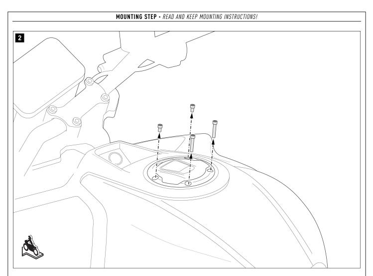
Remove the original screws from the attachment points shown.
