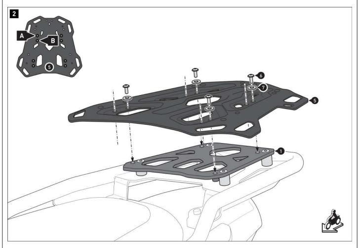
$\triangle$  **NOTE:** Depending on the space available, screw the luggage carrier (5) to the marked mounting position **(A)** or **(B)** as shown in the detailed drawing.
