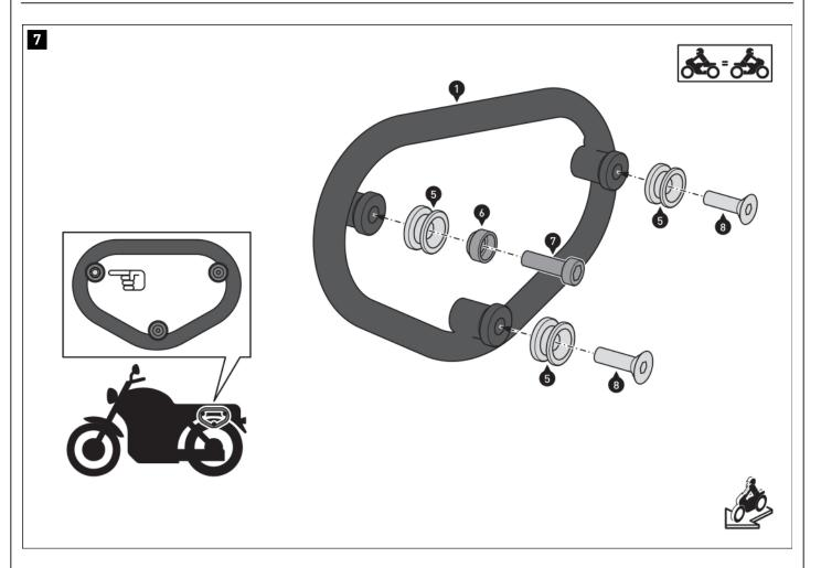
Screw parts (5) to (8) to the side carrier (1). **A** WARNING: Use a liquid threadlocker!
