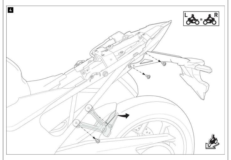
Loosen the original screws, and remove the passenger footrest holder from the bike.
