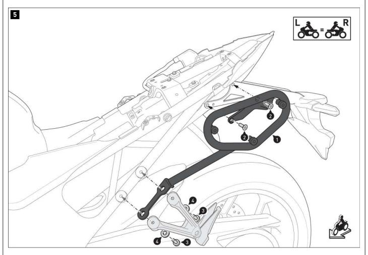
Screw the side carrier (1) to the vehicle. **A WARNING: Use liquid threadlocker!**Tighten screws (2) and (3) according to the bike manufacturer's specifications.
