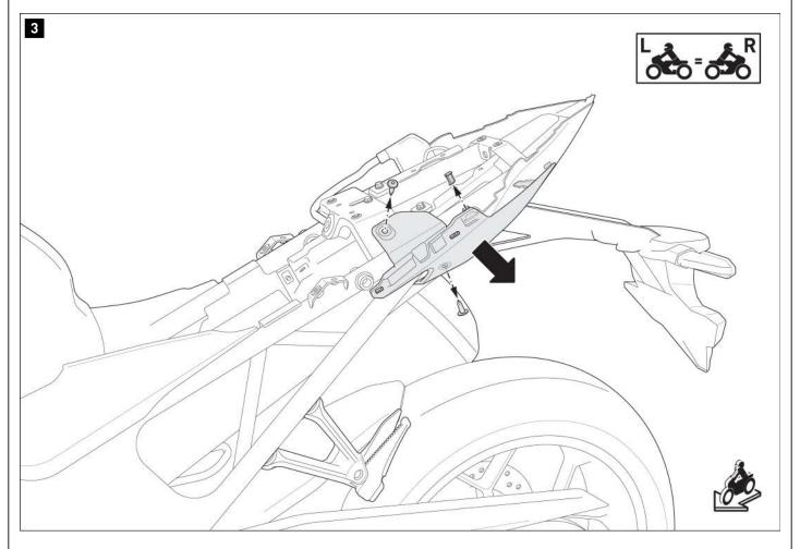
Loosen the original panel dowels, remove the plastic clip, and remove the fairing from the bike.
