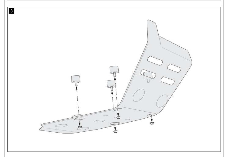
Remove the four rubber dampers from the original engine guard.
