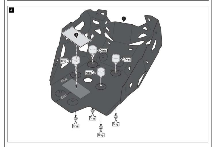
Thoroughly clean the marked surface of the engine guard (1) to remove grease and dirt residues.
