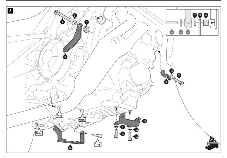
$\triangle$  **NOTE:** The screws (4) and washers (5) are not required if installed at the same time as the SW-MOTECH crash bar. Instead, use the spacer (7) and the parts of the crash bar shown (\*).
