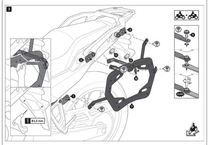
⚠ NOTE: Steps 3 and 4 are optional and can only be carried out with the specified license plate holder. If your vehicle has a different license plate holder, the crossbar (10) is simply fastened between the side carriers (7) and (8) using a Quick-release fastener (9). In this case, no screws are necessary.
