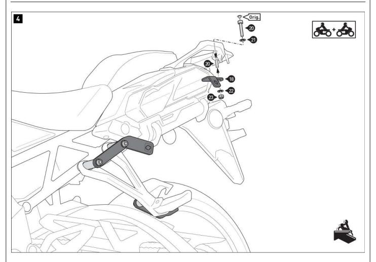
Tighten the screws (20) on both sides of the rack.
