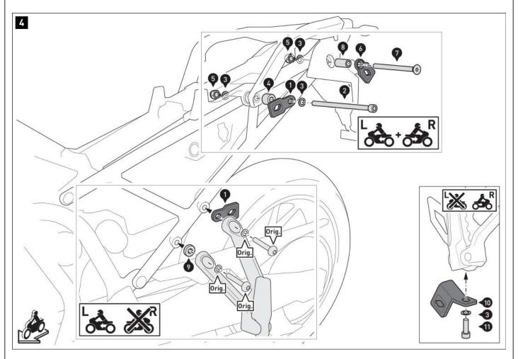
Screw fastening straps (1) and (6) on both sides of the vehicle.
