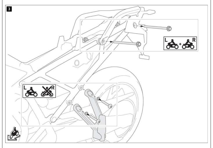
Remove the screws and nuts (as shown in drawing) from both sides of the rear of the vehicle.
