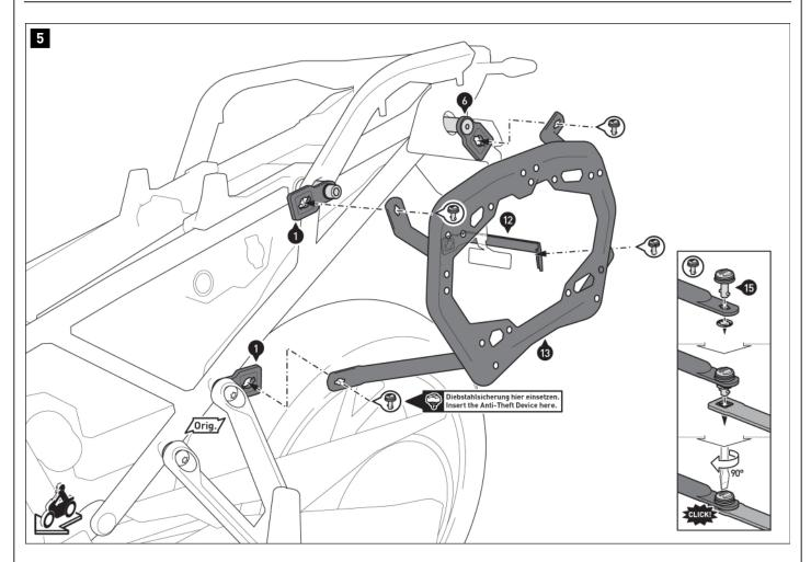
$\triangle$  **NOTE:** The SW-MOTECH anti-theft protection devices are available separately; mount the anti-theft protection devices on both sides at the marked position.
